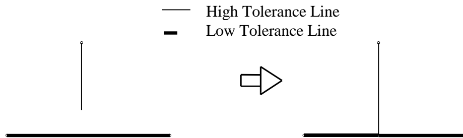
Figure 19: Fuzzy intersection created in linear feature with smaller tolerance
